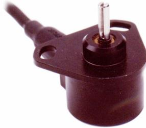
The output of a rotary potentiometer is a voltage which changes in direct proportion to the shaft angle. A constant voltage is required across the supply and ground wires of the sensor. No internal end stops are fitted, so continuous rotation is possible. The sensors are fully sealed against the ingress of fluids. Various lengths of electrically active track are available, up to a maximum of 348°.
